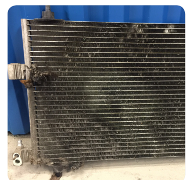
Seems tight, however, a condenser in such a condition cannot perform well and must definitely be replaced
