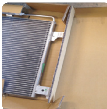
Poor quality packaging cannot ensure a proper damage protection during transportation and storage
