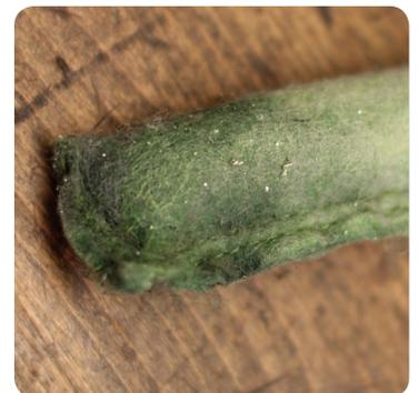
Worn out insert bag dryer - desiccant soaking by too much UV agent added to the system
