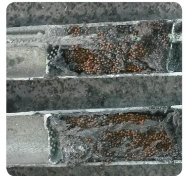
Worn out desiccant and filtering layers inside the receiver dryer
