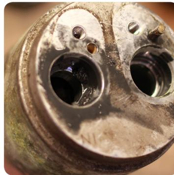
Contamination of the in- and outlets will cause the receiver dryer to clog
