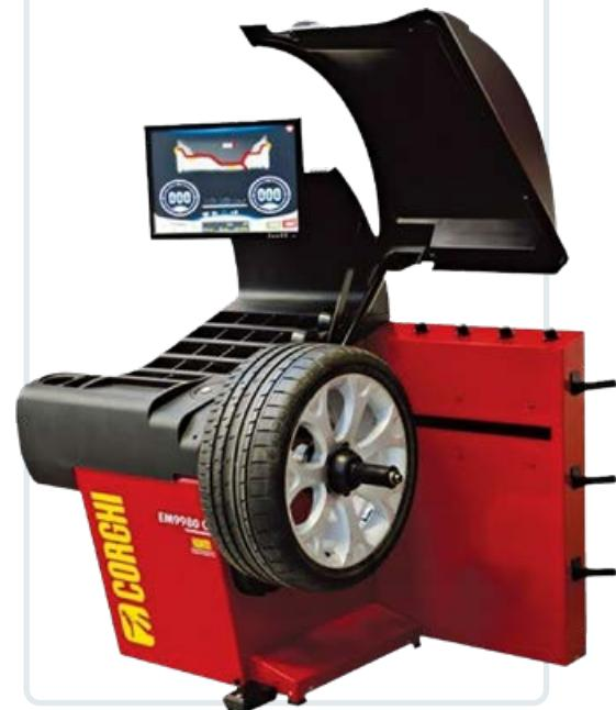
**UREĐAJ ZA BALANSIRANJE KOTAČA
